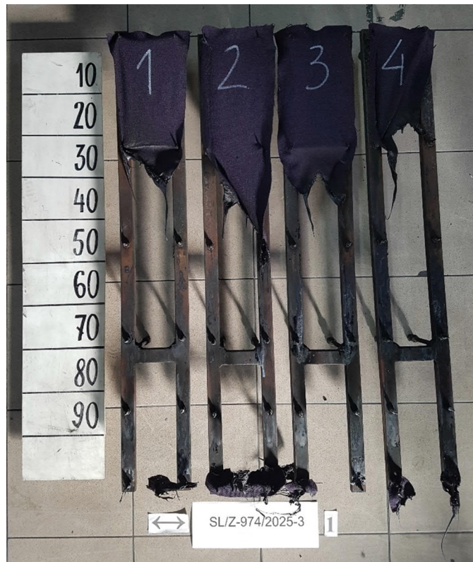
Figure 3. Appearance of the sample 2 after the test – Aubergine D1644D, cross direction
