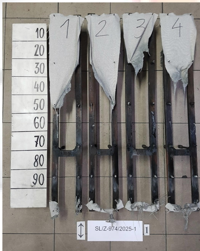
Figure 4. Appearance of the sample 3 after the test – Light Grey D1644C, length direction
