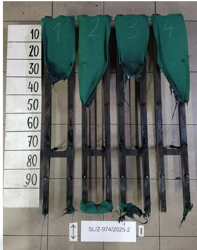
Figure 5. Appearance of the sample 4 after the test – Green D1644B, length direction
