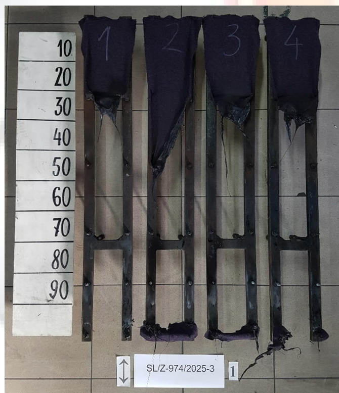
Figure 2. Appearance of the sample 1 after the test - Aubergine D1644D, length direction
